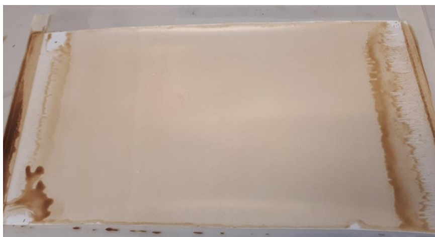
FIGURE 2.6 EXAMPLE OF A LARGE-AREA SUPPORTED GO MEMBRANE
