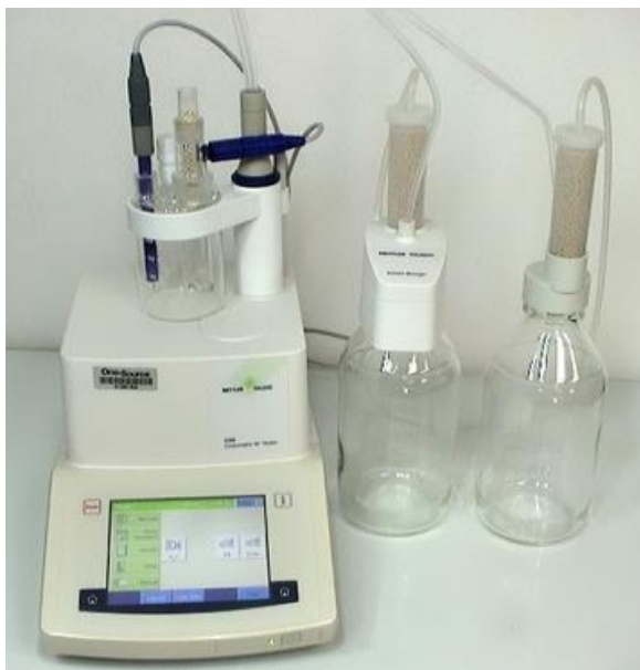
FIGURE 2.7 C20 METTLER TOLEDO AUTOMATIC TITRATOR
